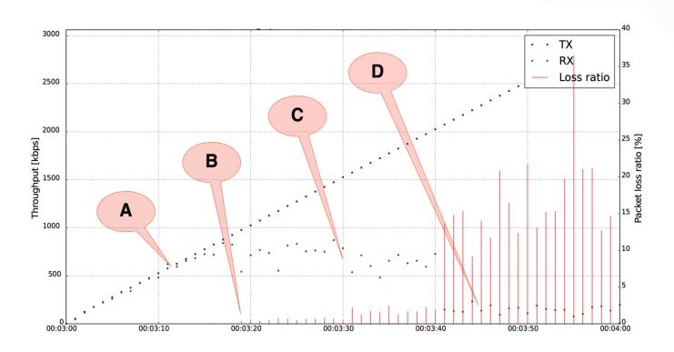
Point **A** indicates the area of initial saturation of the data link. Point **B** shows the moment of the first recorded loss of packet. Point **C** is in the area of maximum data link throughput before significant loss of packets begins. A heavily congested data link is the area around the **D** point.
