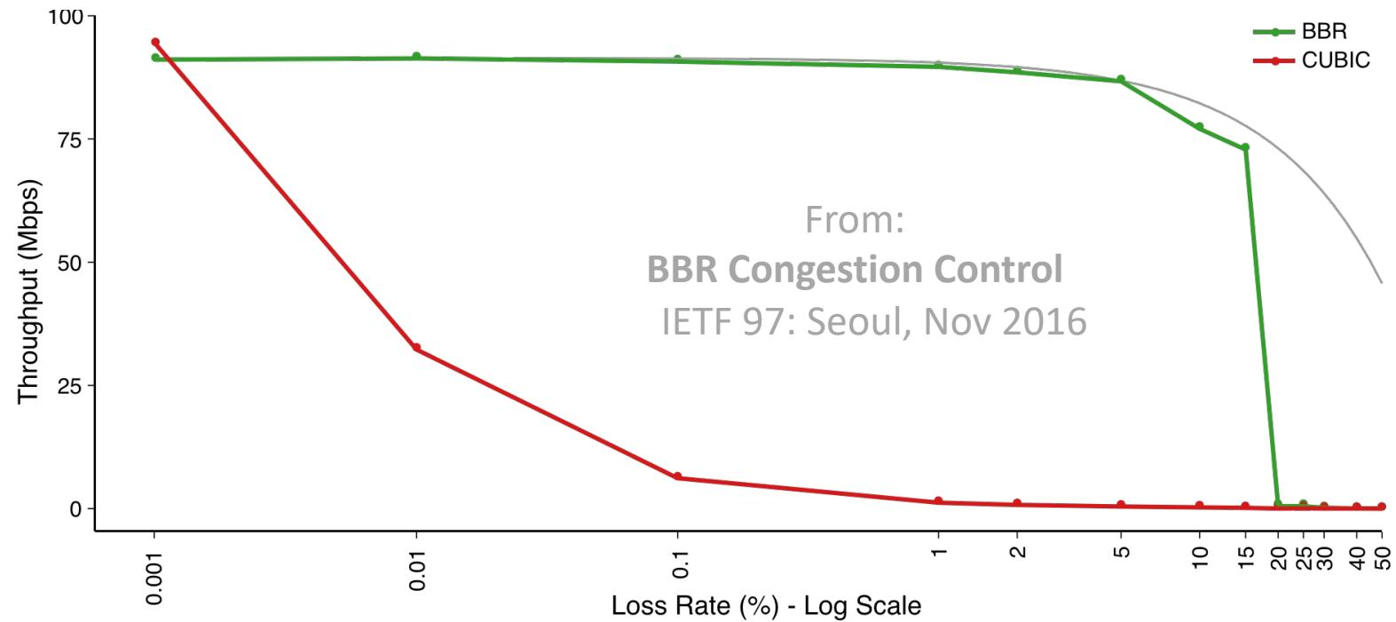
BBR vs CUBIC: synthetic bulk TCP test with 1 flow, bottleneck\_bw 100Mbps, RTT 100ms
